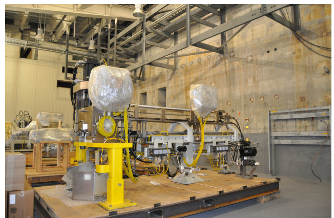
The rocket shear machine (RSM) which will punch and drain the warhead then shear it into multiple pieces for processing in the energetics batch hydrolyzer (EBH), is staged in the MDB
