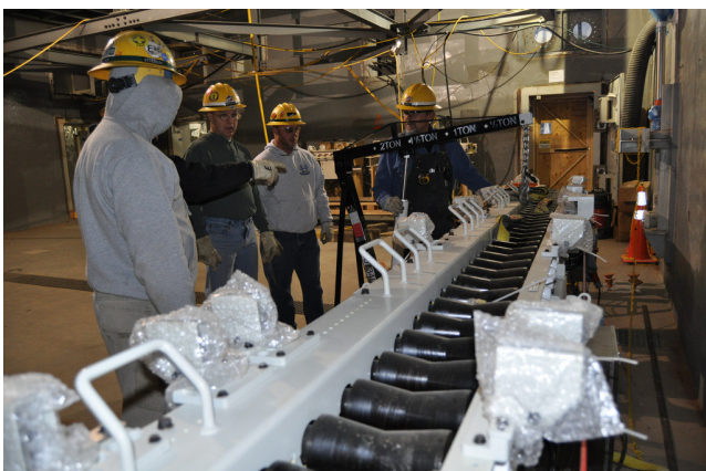
Conveyors are used to transfer the chemical weapons to various stations in the munitions demilitarization building (MDB)
